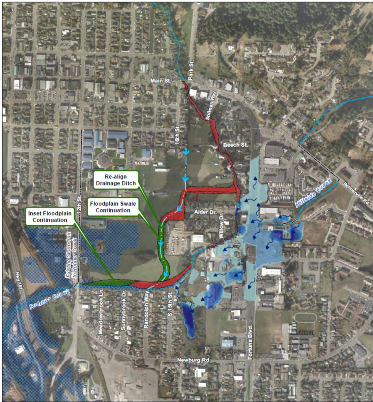
Figure 3. Rohner Creek Phases and 100- year Flood after Completion of Phases 1 and 2 (Currently Under Construction)
